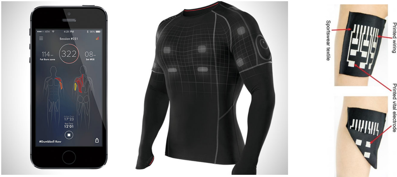
Example of textile sensor to detect muscle activity.
