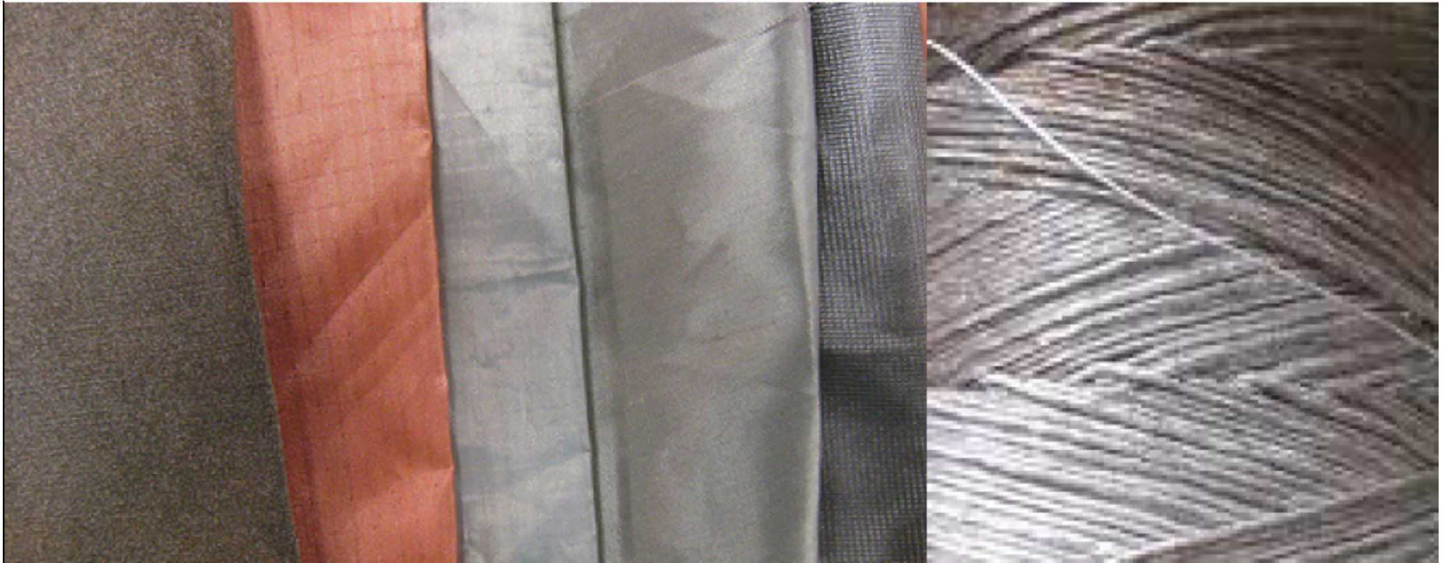
Conduct Electricity: Textile and Yarn able to conduct electricity
